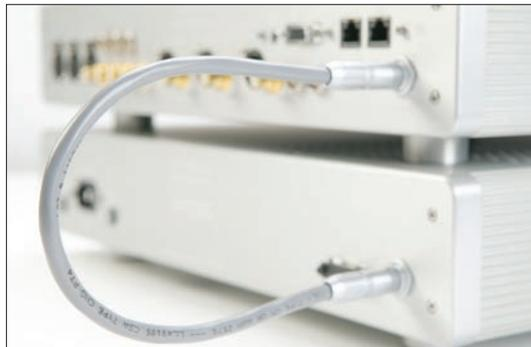
Above: Evolution Two inputs labelled only as S1-4, B1-3 and C1-3 on the panel (single-ended/balanced/CAST), but can be assigned pre-set names for the fluorescent display like 8TRK, DCC, GAME and HI-8; [left] unlike power amp, power connection from PSU to pre-amp is by cable
